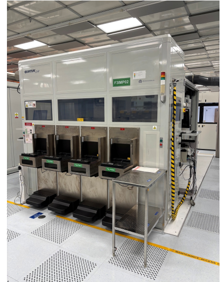
Quantum LEAP implanter in a 200mm fab, with front-end load ports
